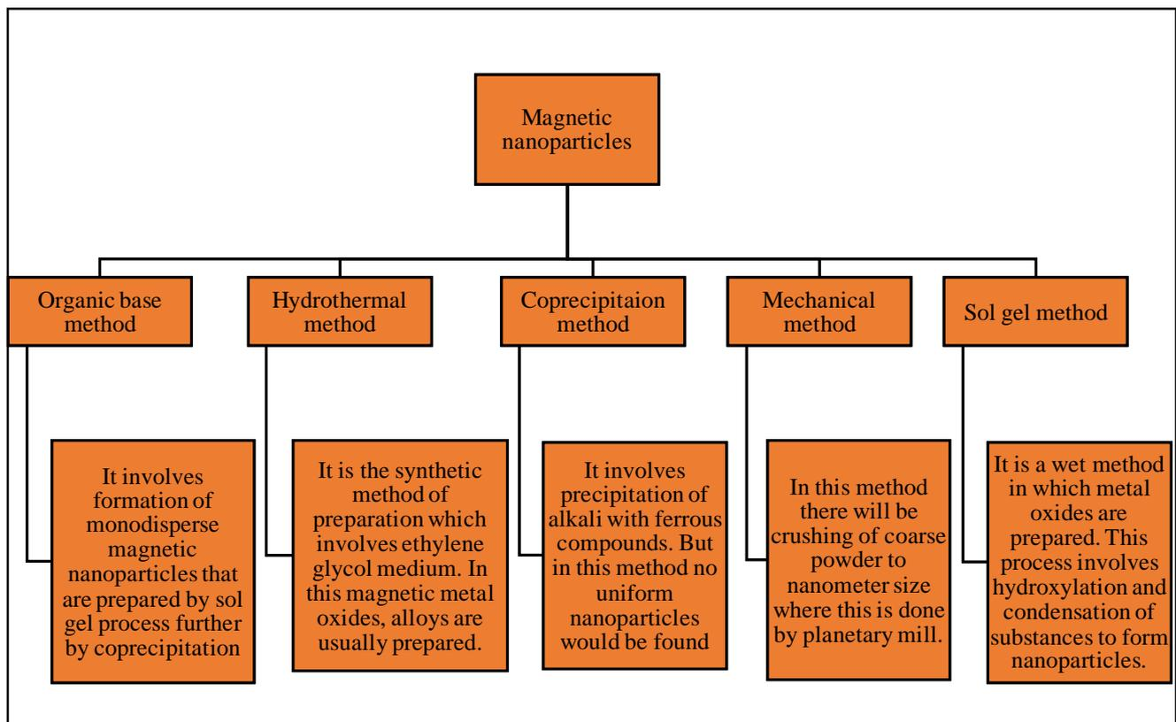
**Figure 2: Method of preparation of MNPs, 1. Organic base method; 2. Hydrothermal method; 3. Coprecipitation method; 4. Mechanical method; 5. Sol-gel method.**
